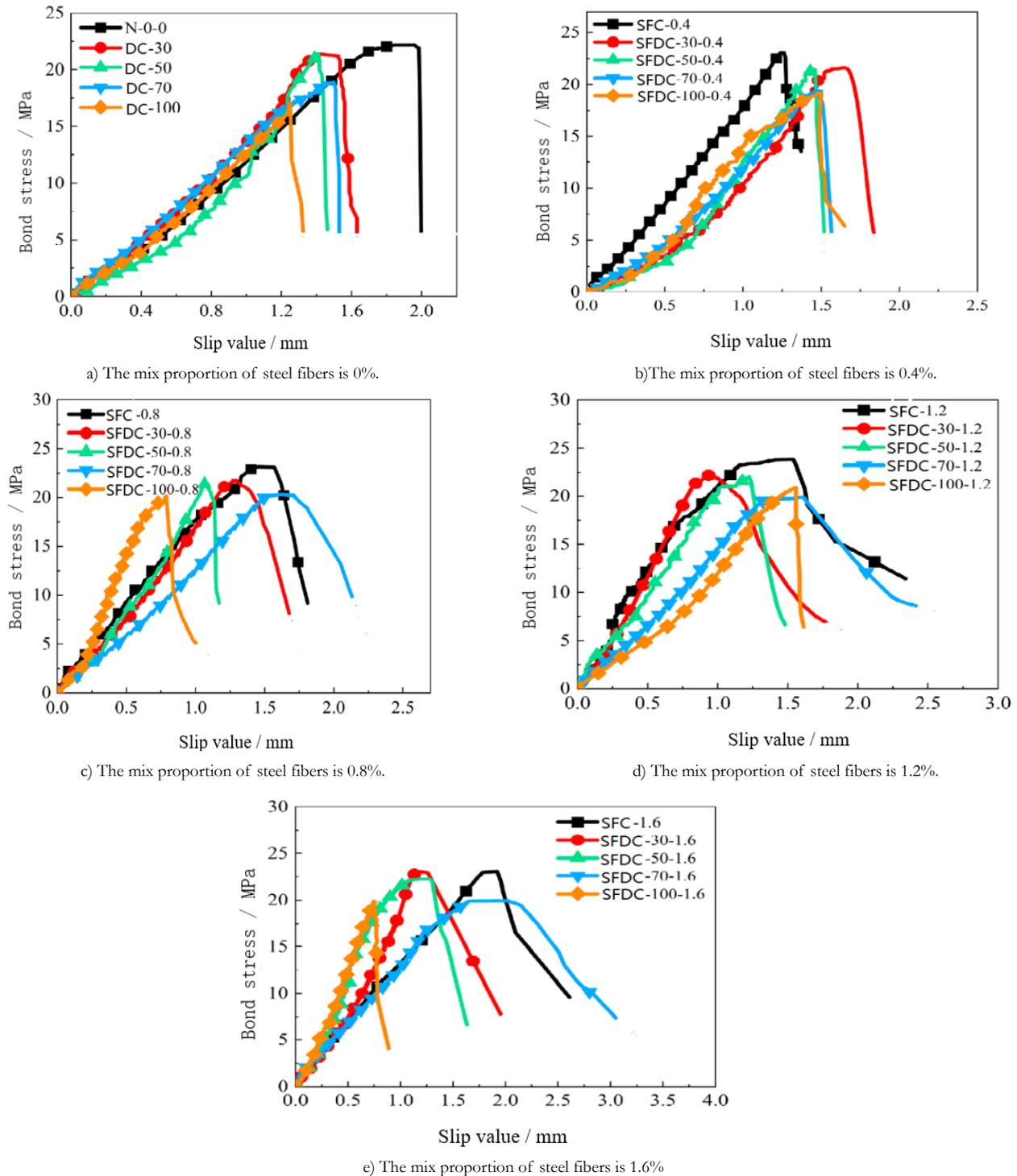
Figure 4: The bond stress-slip relationship curve under different replacement rates of recycled aggregates.
