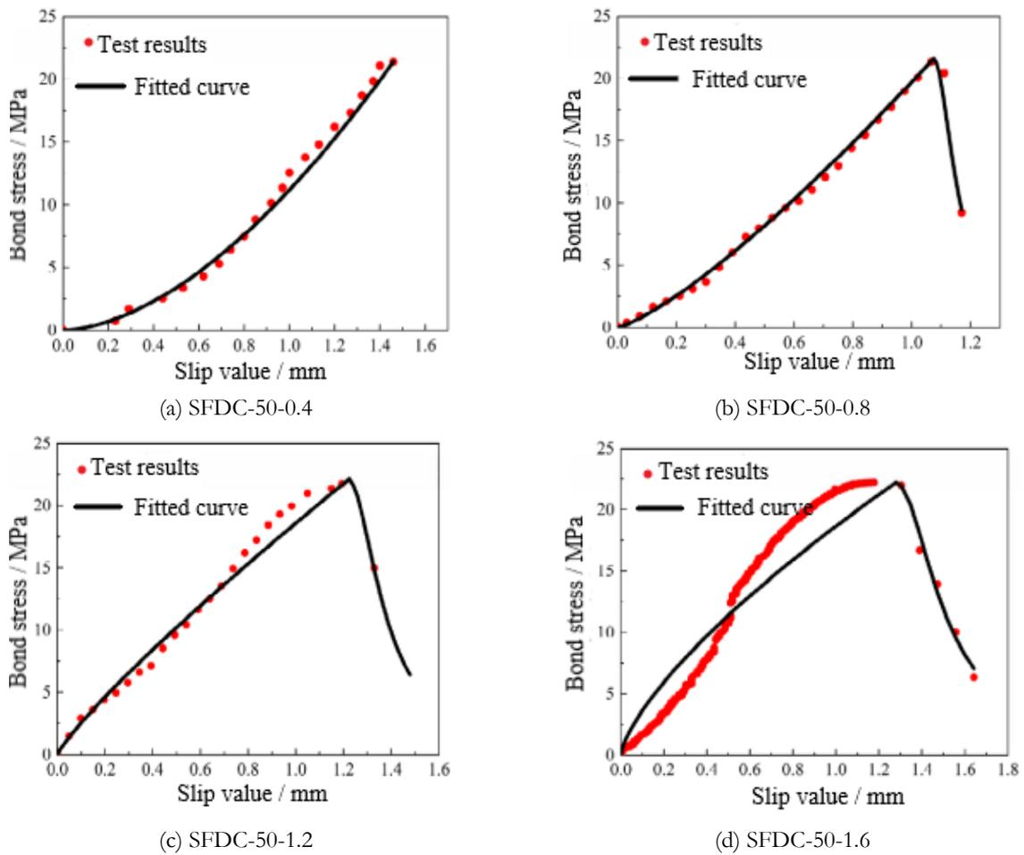
Figure 7. The test curves and fitted curves.
