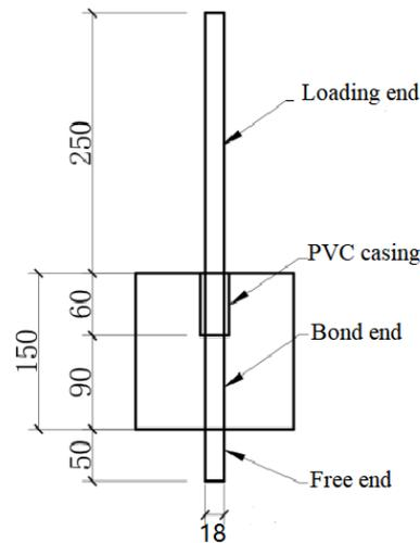
Figure 1. The design dimensions of the test specimen (unit: mm)
