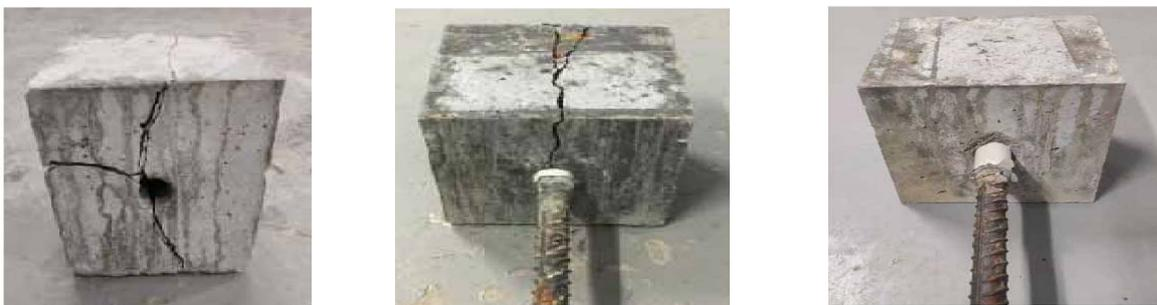
(a) Splitting failure      (b) Splitting pull-out failure      (c) Pull-out failure
