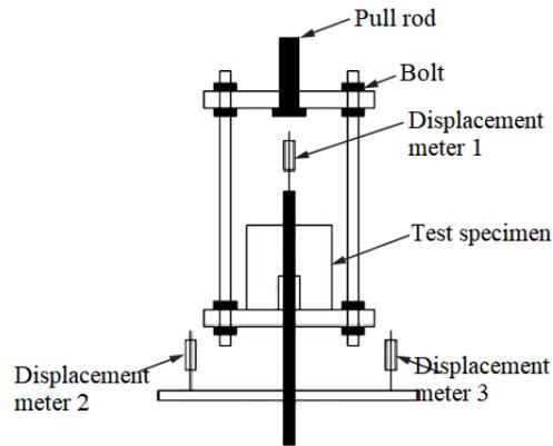
Figure 2. The layout drawing of the loading device
