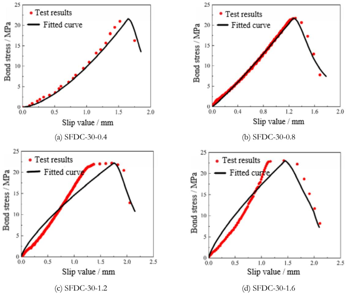
Figure 6: The test curves and fitted curves.
