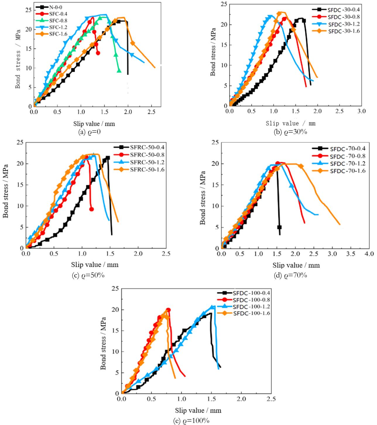
Figure 5: The bond stress-slip curve under different mix proportions of steel fibers.
