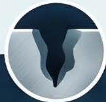
Lack of Penetration (LOP)
