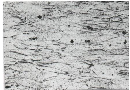
Figure 4c: “4L” steel microstructure - Radial section (x 200).
