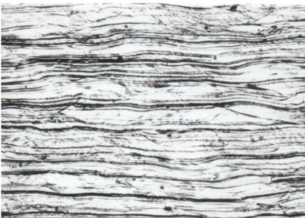
Figure 4a: “4L” steel microstructure - Longitudinal section (x 200).
