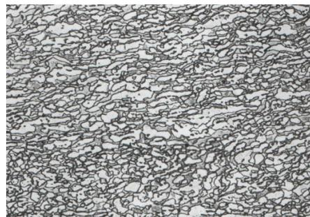
Figure 2b: “A1L” steel microstructure - Transversal section (x 200).
