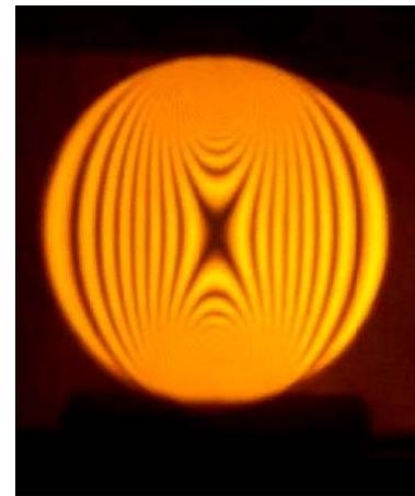
Figure 5. Isochromatic fringes in calibration disk.
