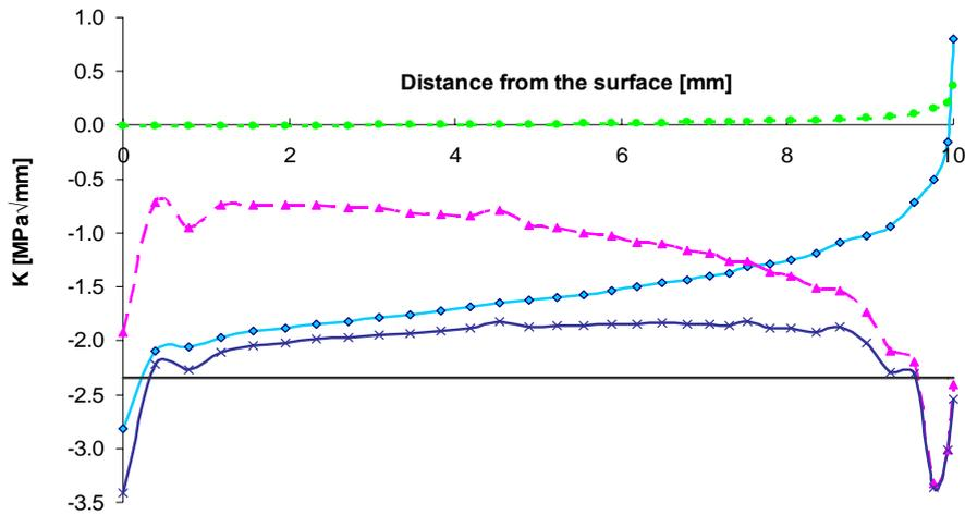
Figure 10. Stress intensity factors along the crack front in function of the depth. (—●—  $K_I$ , —◆—  $K_{II}$ , —▲—  $K_{III}$ , —×—  $K_{IIeq}$ , —  $K_{II-2DFEM}$  [10]).
