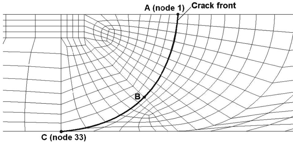
Figure 8. Meshing configuration around the curved crack tip.
