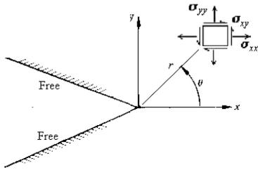
Figure 1. Crack tip coordinates and stress components.
