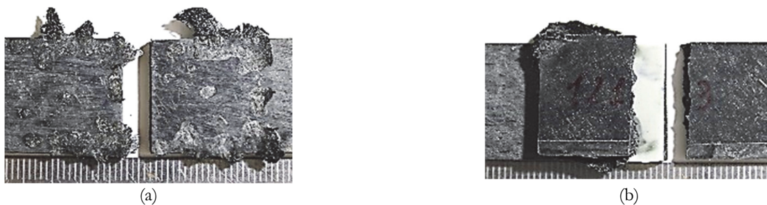
Figure 3: The OM images of the fractured USW-joints: along the fusion zone (by the interlayer shear mechanism) without EDs at t_{USW}=1000 ms (a) and along the base material (cohesive fracture due to bending) at \delta=100 μm and t_{USW} =1000 ms (b); USW mode #1
