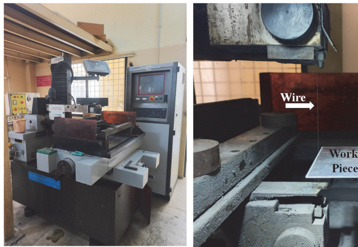
Figure 7: Wire EDM equipment and setup.
