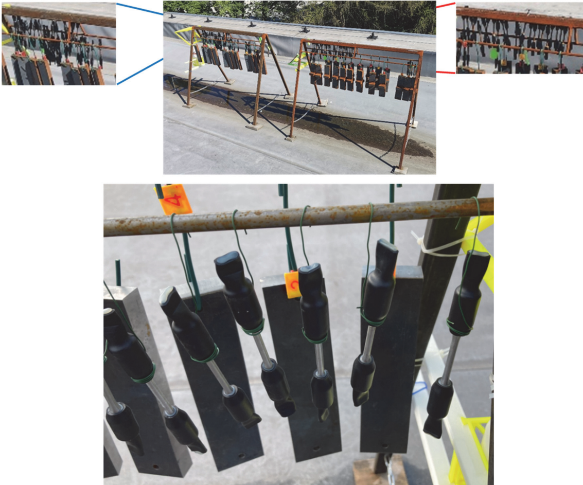
Figure 4. S460NL fatigue specimens exposed to natural atmospheric conditions on the roof of the Experimental and Diagnostic Building Center at VŠB–TU Ostrava. The specimens were mounted on an outdoor exposure frame to simulate real environmental conditions. Plastic covers were used to protect the threaded ends of the specimens from corrosion.
