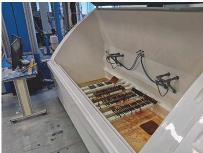
Figure 3. S460NL fatigue specimens placed inside the Ascott S2000is corrosion chamber during the accelerated salt spray corrosion test according to ISO 9227. The specimens correspond to the corrosion exposure groups of 3 days (35°C), 6 days (35°C), and 6 days (35°C) + 3 days (50°C). Plastic covers were used to protect the threaded ends of the specimens from corrosion.
