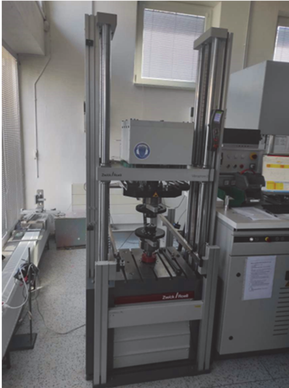
Figure 6. Experimental set up for fatigue: ZwickRoell Vibrophore resonance pulsator with specimens.
