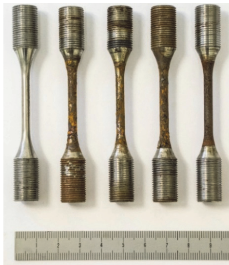
Figure 5. Examples of steel specimens for fatigue experiments without and with four various levels of corrosion. Reference; 3 (35°C) days; 6 (35°C) days; 6 (35°C) +3 (50°C) days specimens and specimen from natural exposure (from left to right).
