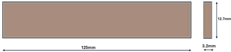
Figure 2: Dimensions of the flexural test specimen.
