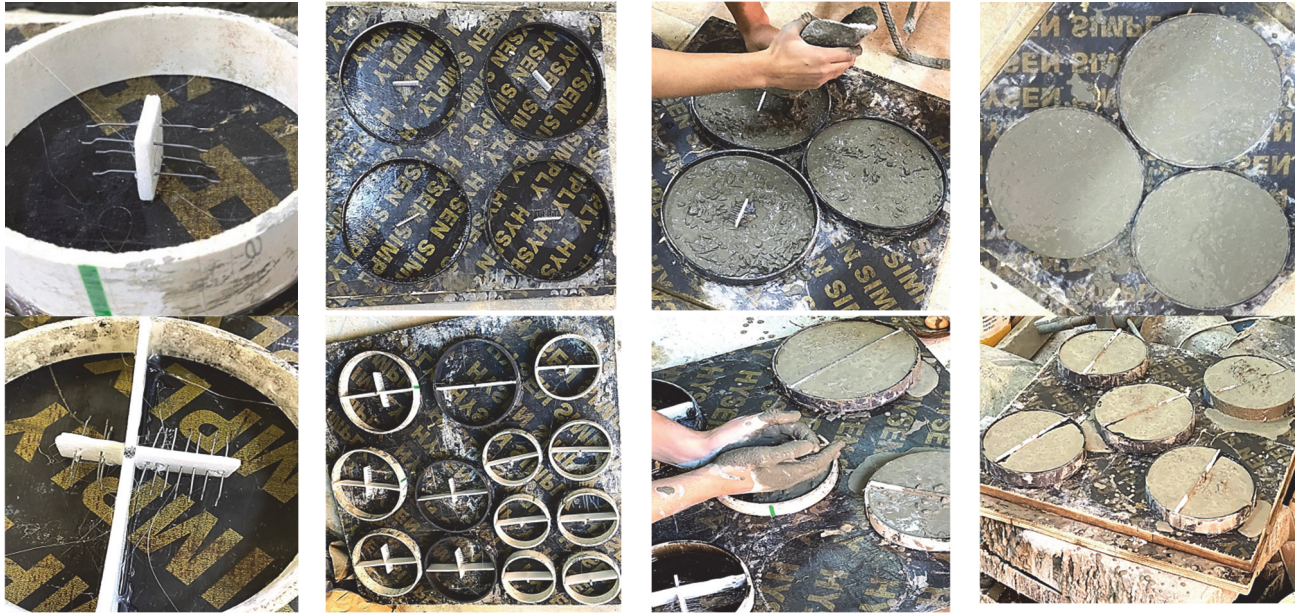
Figure 1: The main steps of preparing and casting of CCCD and SCB specimens.
