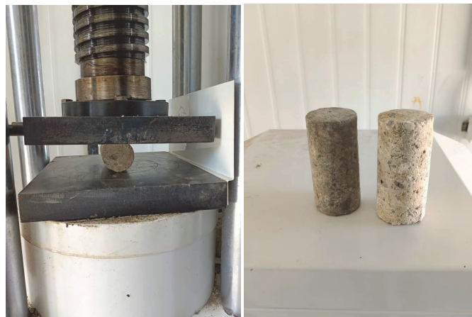
Figure 12: Splitting tensile Test.
