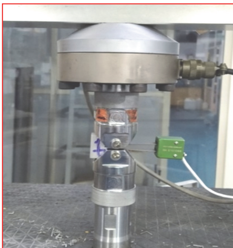
Figure 9: Testing using a servo-hydraulic universal testing machine.
