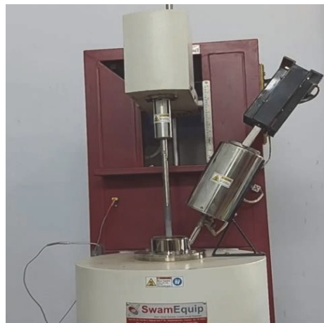
Figure 7: Experimental set up of stir casting equipment.
