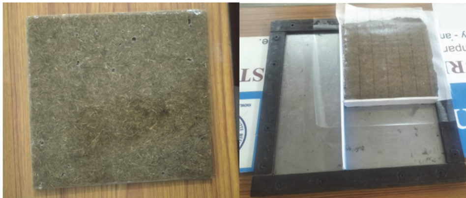
Figure 1: Composites specimen slab and preparing the composite specimens.
