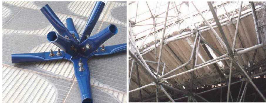
Figure 1: Connection configuration of the end-flattened steel bars (a) and the collapse of a three-dimensional truss (b) [1].
