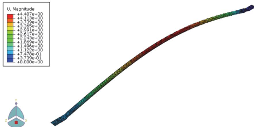
Figure 14: Displacements referring to the global buckling of a numerical model example in Abaqus® software, in millimeters (mm).
