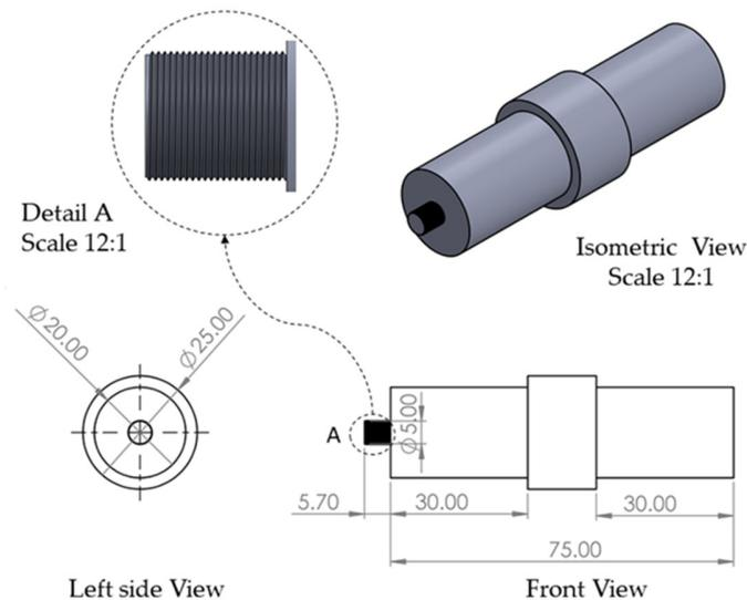
Figure 3: Friction Stir Welding Tool Design used in the present work
