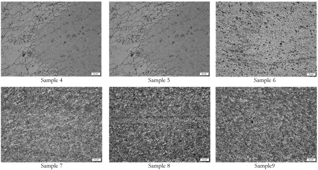
Figure 8: Microstructure images of Stir Zone.
