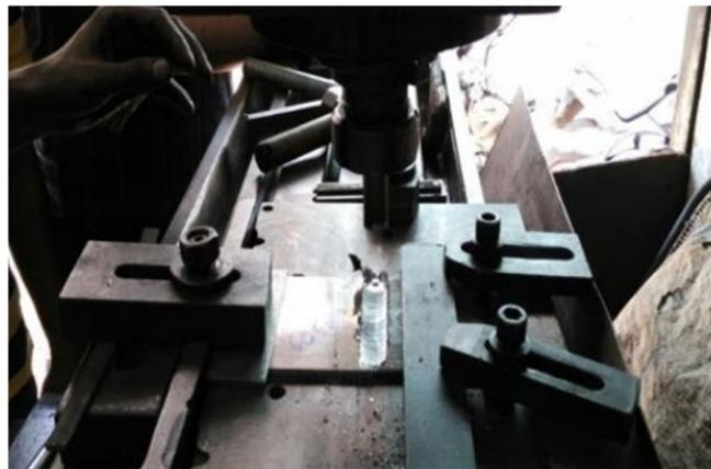
Figure 2: Friction Stir Welding process setup
