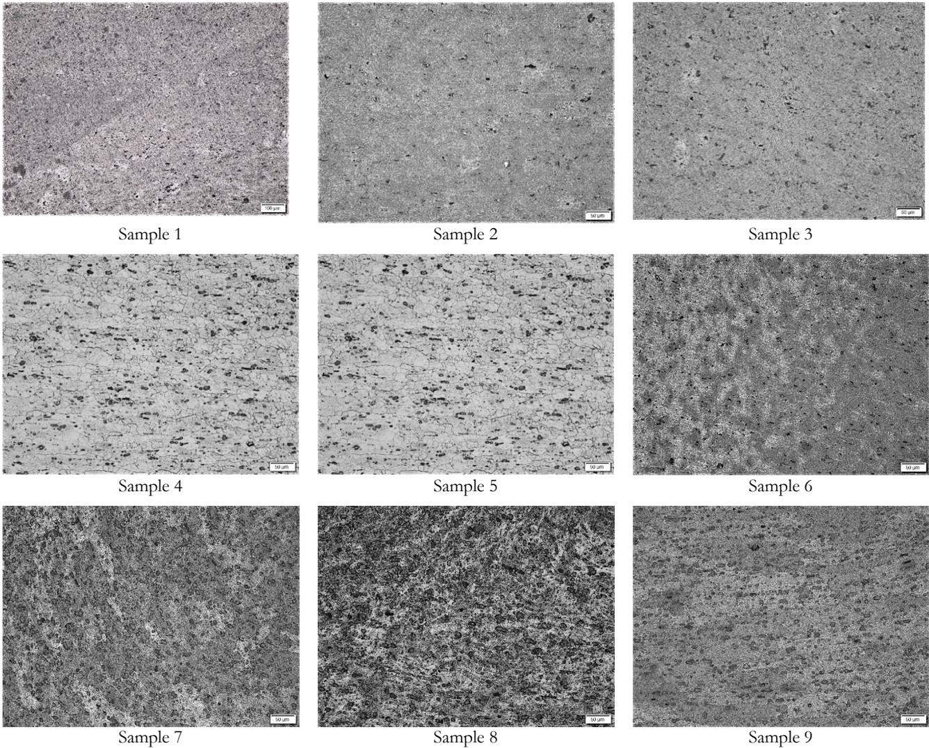
Figure 7: TMAZ Microstructures.
