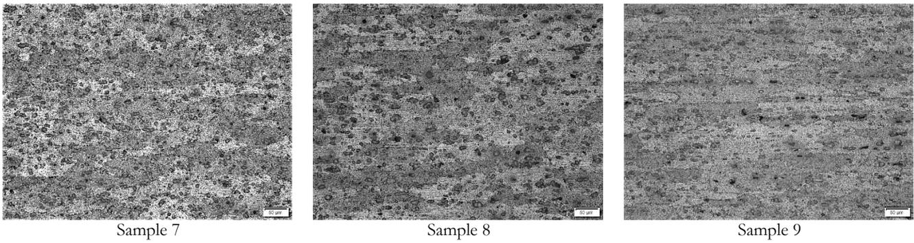
Figure 9: Microstructure images of Heat Affected Zone.
