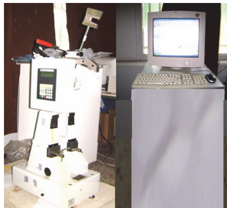
Figure 2: Zwick/Roell type Charpy impact machine used.
