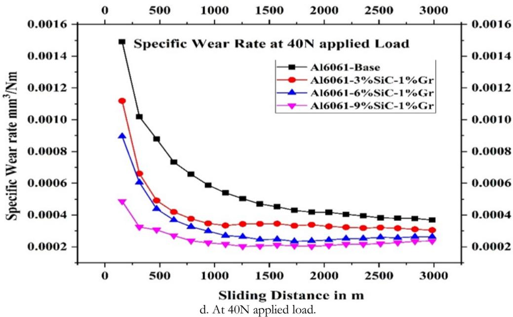
Figure 9: a-d. The specific wear rate of Al6061 Alloy and SiC- Gr MMCs with a 3.0 km sliding distance at 10 – 40 N loads.
