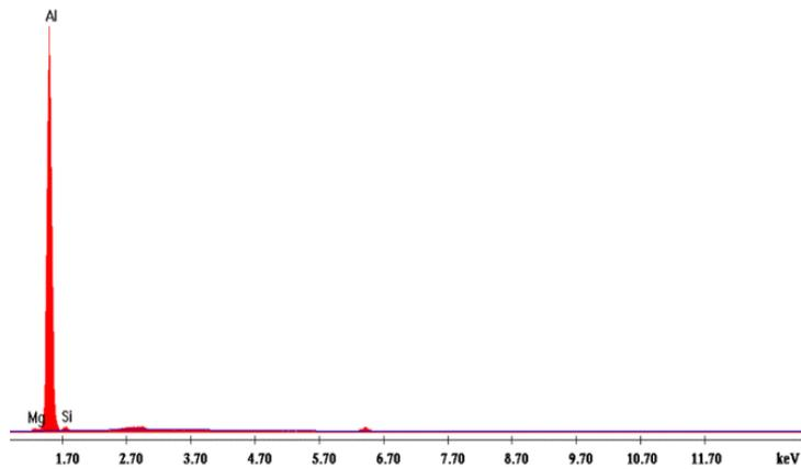
Figure 1: EDX image of Al6061 matrix alloy.
