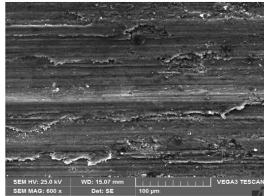
d. SEM of worn-out Al6061-9wt% SiC.
