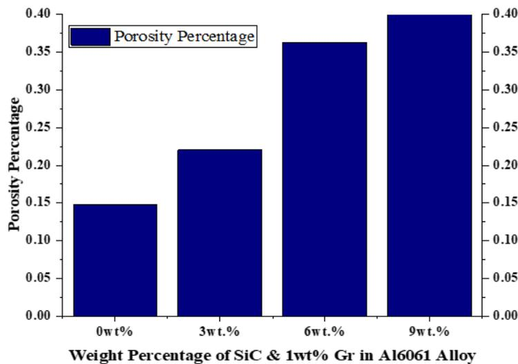
Figure 4: Variation in Porosity of Al6061-SiC-Gr HMMCs.
