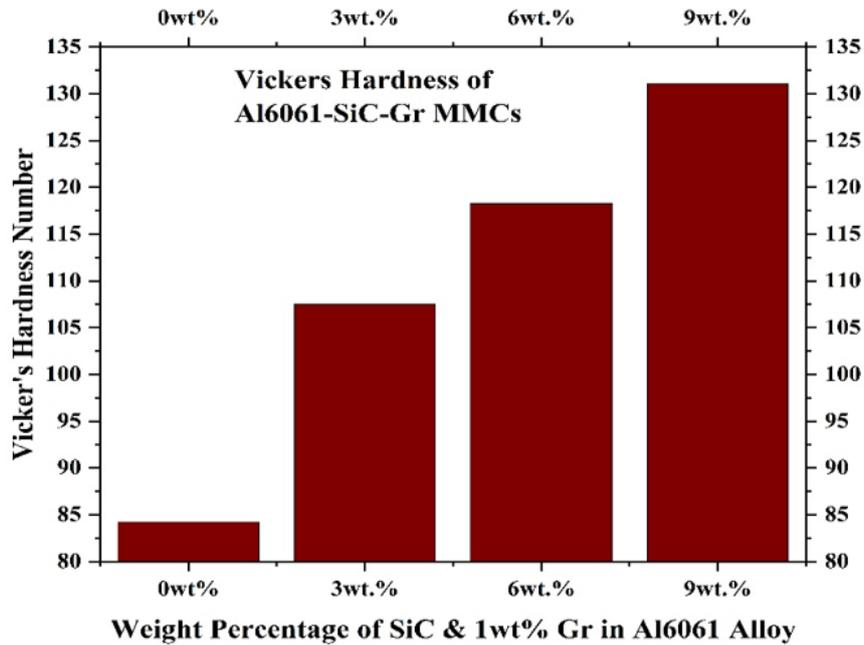
Figure 5: Hardness values of Al6061-SiC-Gr HMMCs.
