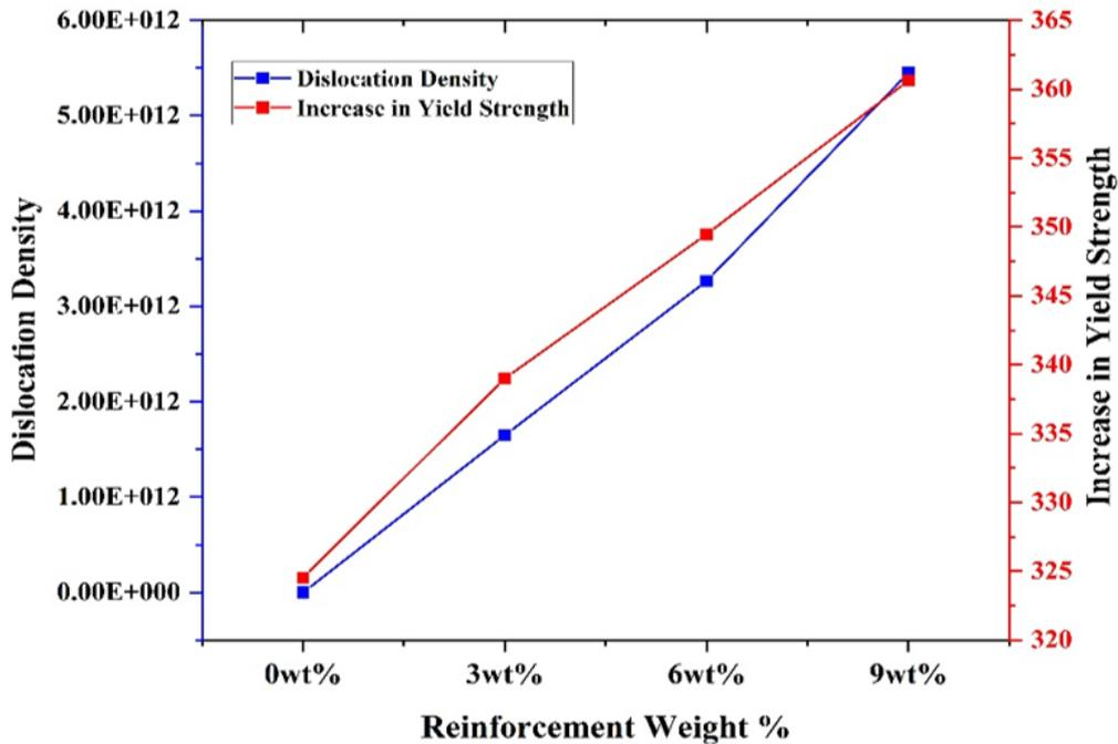
Figure 6: Dislocation Density and Increase in Yield strength of Al6061-SiC-Gr HMMCs.
