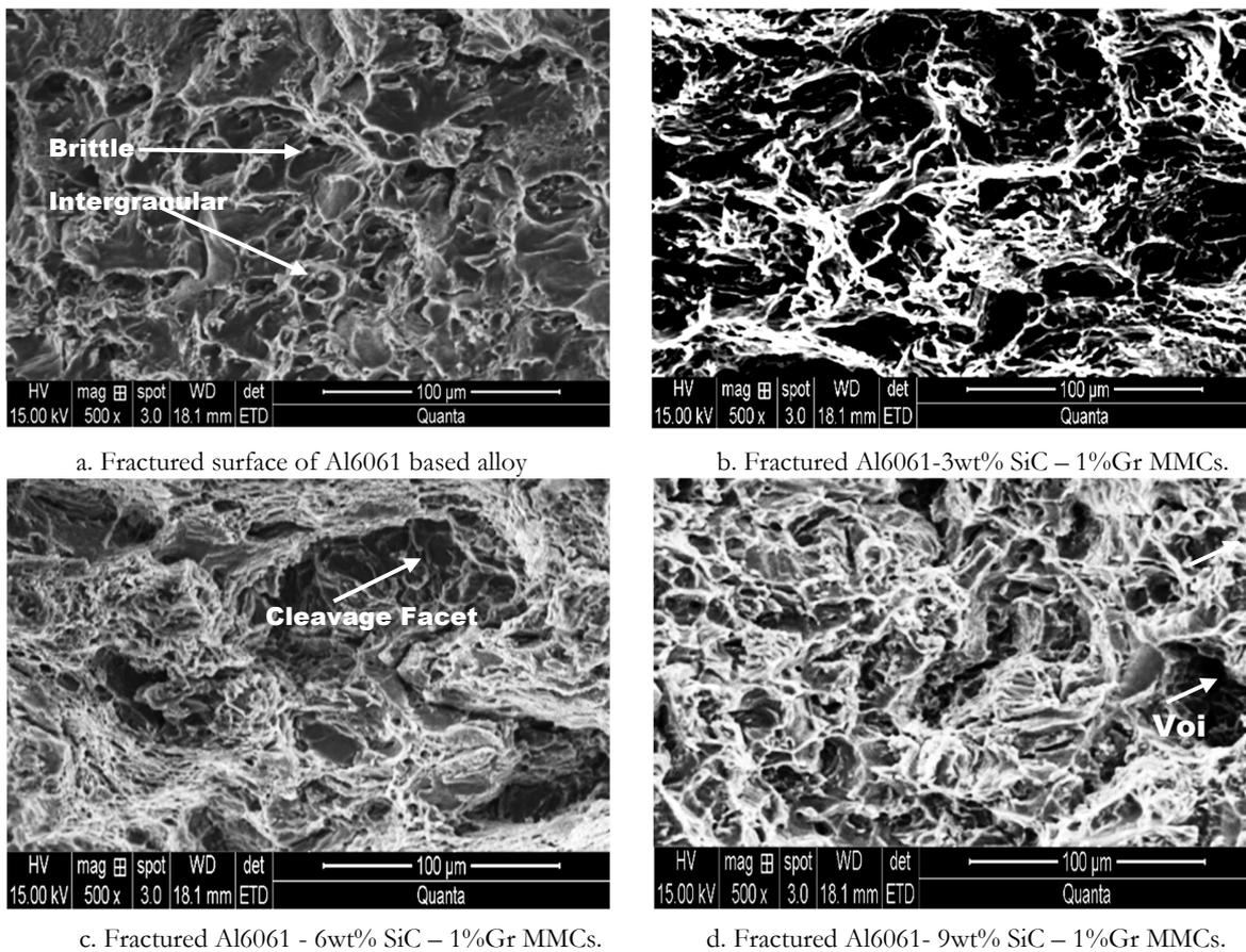
Figure 8: a-d. SEM micrographs of tensile test fractured sides of Al6061 and Al6061- SiC - Gr HMMCs.
