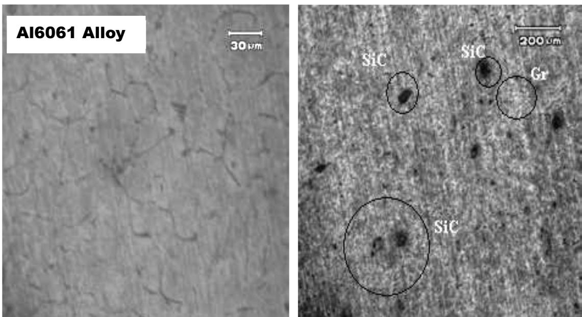
Figure 2: Optical micrograph of (a) Al6061 alloy, (b) MMC (Al6061-9wt.% SiC-1wt.% Gr).
