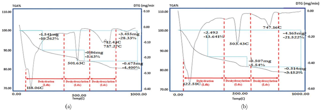
Figure 13: TGA/DTG of cement paste of the control at the ages of (a) 28 days and (b) 90 days.
