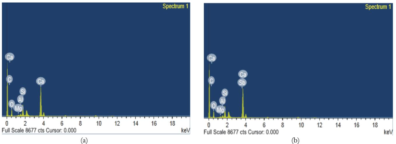
Figure18: (a) EDS (X-ray) analysis of the mix(1) 100% OPC mix at 90 days and (b) EDS (X-ray) analysis of the mix(5) 100% OPC of 150 Cycles of magnetized water at 90 days.
