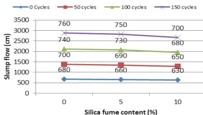
Figure 5: Slump flow of SCC mixes with or without Silica fume modified with magnetized water or regular tap water.
