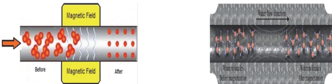
Figure 1: Effect of magnetic field on water clusters [7, 8].
