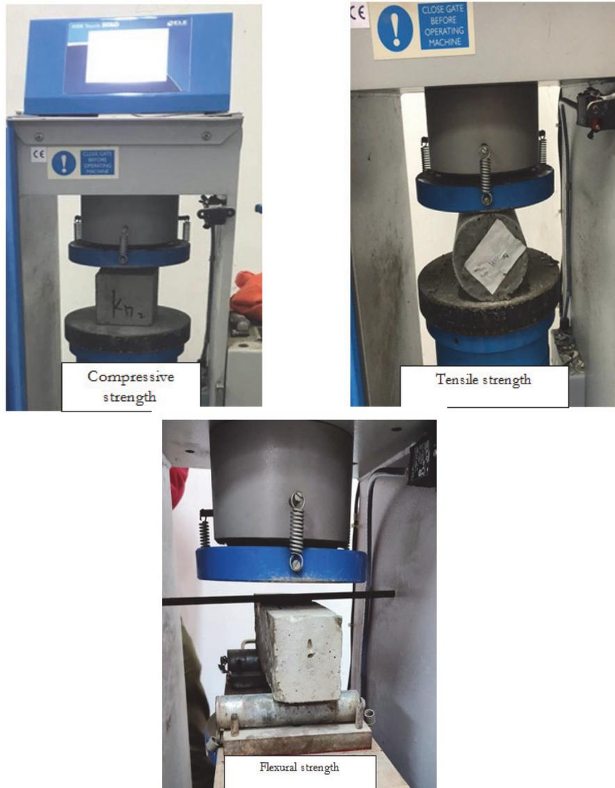
Figure 4: Hardened properties Tests.
