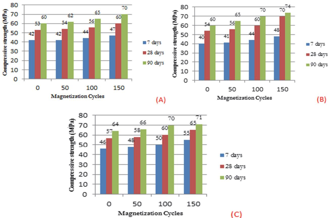
Figure 9: Compressive strength of SCC mixes with (a)0%, (b)5%and (c)10% Silica fume prepared with magnetized water and tap water.
