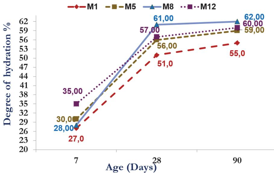
Figure 12: Hydration degree assessment of cement paste.
