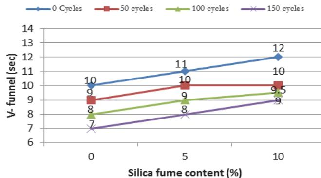
Figure 7: V-funnel test of all SCC mixes with or without Silica fume modified with magnetized water or regular tap water.
