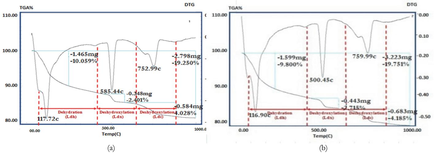
Figure 15: TGA/DTG of cement paste of 5% SF with 150 cycles of MW at the ages of (a) 28 days and (b) 90 days.
