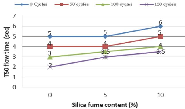
Figure 6: T50 results of SCC mixes with or without Silica fume modified with magnetized water or regular tap water.
