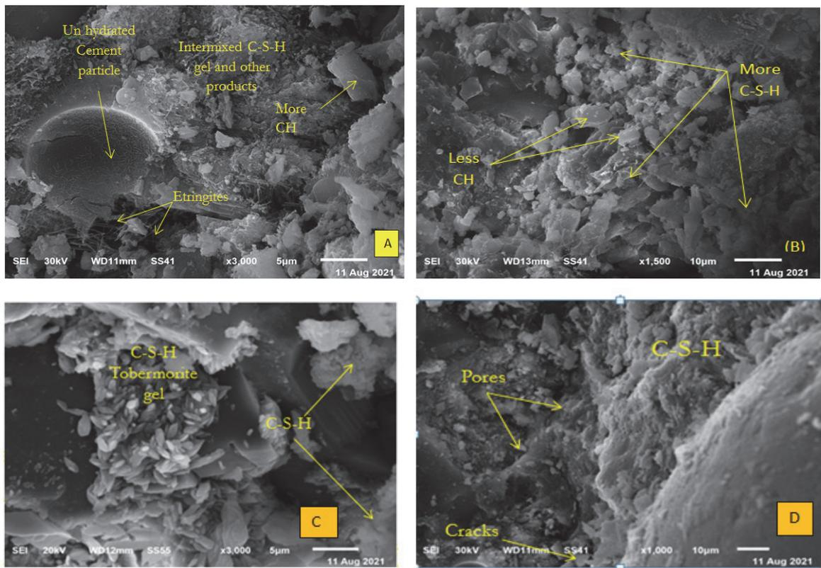
Figure 17: SEM images for (A) SEM image for the 100% OPC Mix1 at 90 days, (B) SEM image for the 100% OPC + 150 Cycles of magnetized water Mix5 at 90 days, (C) SEM image for Mix(5) the 100% OPC + 5% silica fume + 150 Cycles of MW at 90 days and (D) SEM image for the Mix(D) 100% OPC+ 10% silica fume+ 150 Cycles of MW at 90 days.
