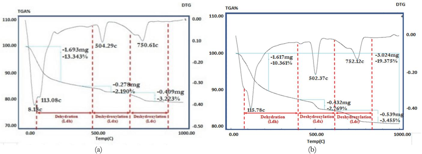
Figure 16: TGA/DTG of cement paste of 10% SF with 150 cycles of MW at the ages of (a) 28 days and (b) 90 days.
