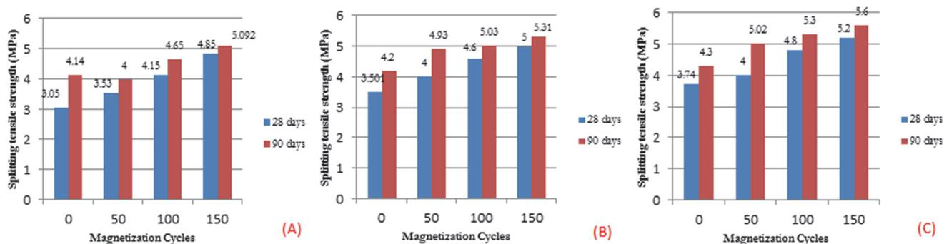
Figure 11: Splitting tensile strength of SCC mixes with (a) 0%, (b) 5% and (c) 10% Silica fume prepared with magnetized water and tap water.
