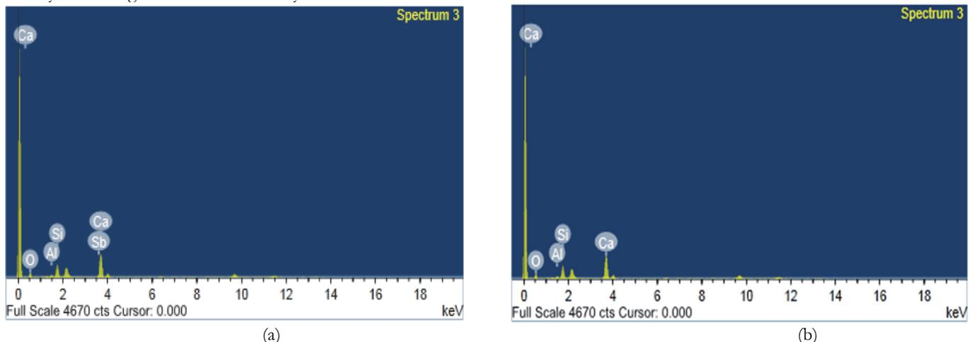
Figure19: (a) EDS (X-ray) analysis of the mix (M8)100% OPC+ 5% Silica fume mix with 150 Cycles of magnetized water at 90 days(b) EDS (X-ray) analysis of the mix(M12) 100% OPC+ 10% Silica fume mix with 150 Cycles of magnetized water at 90 days.
