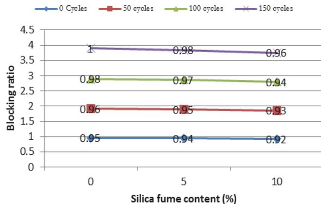
Figure 8: L-box test of all SCC mixes with or without Silica fume modified with magnetized water or regular tap water.
