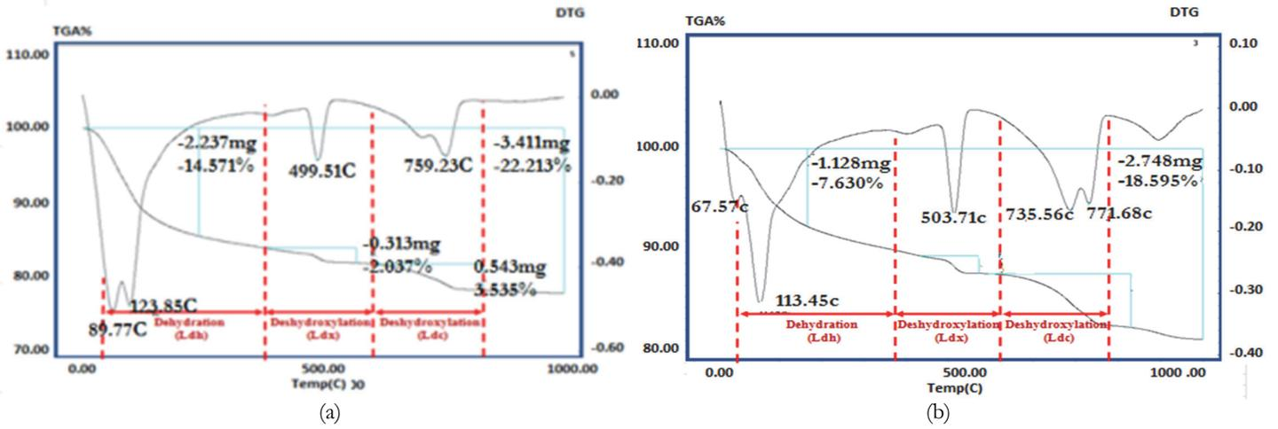
Figure 14: TGA/DTG of cement paste of the control with 150 cycles of MW at the ages of (a) 28 days and (b) 90 days.
