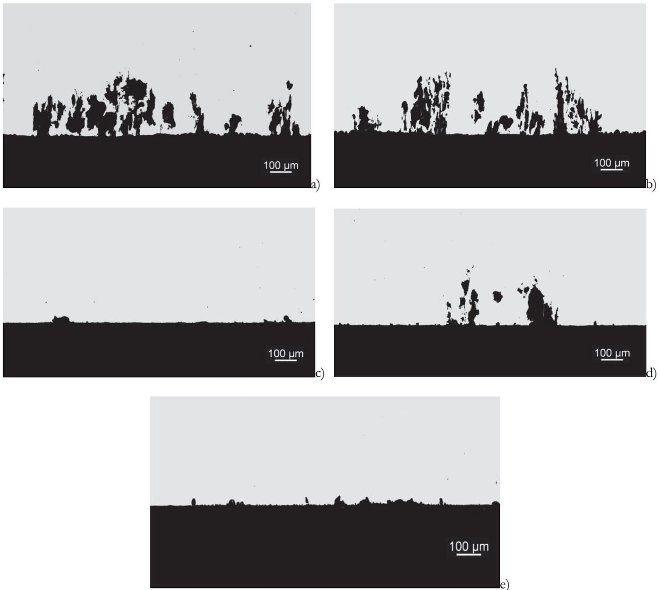
Figure 7: Results of intergranular corrosion tests in samples with different ageing parameters – a) 121°C, 24h; b) 140°C, 12h; c) 140°C, 81h; d) 166°C, 3h; e) T76.
