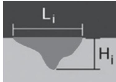
Figure 1: Image analysis of a corrosion pit.
