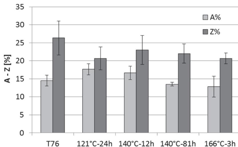
Figure 6: Comparison between the percentage elongations (A%) and the reductions of area (Z%).
