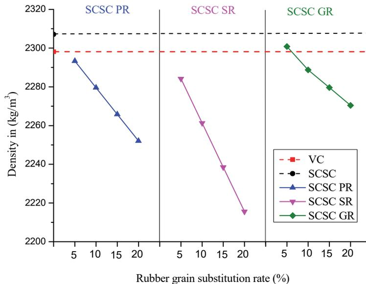
Figure 10: Concretes densities (in kg/m<sup>3</sup>) evolution vs. rubber substitution rate (in %)
