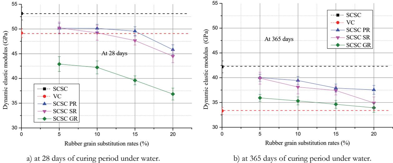
Figure 11: Dynamic elastic modulus variation (in GPa) for concrete samples vs. rubber content.
