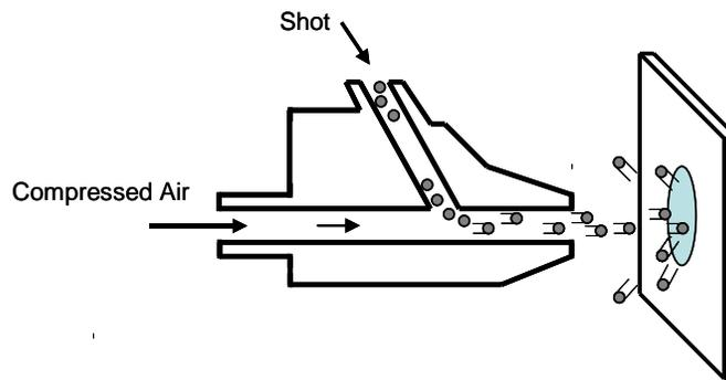
Figure 3: Schematic illustration showing the equipment of ABSP.
