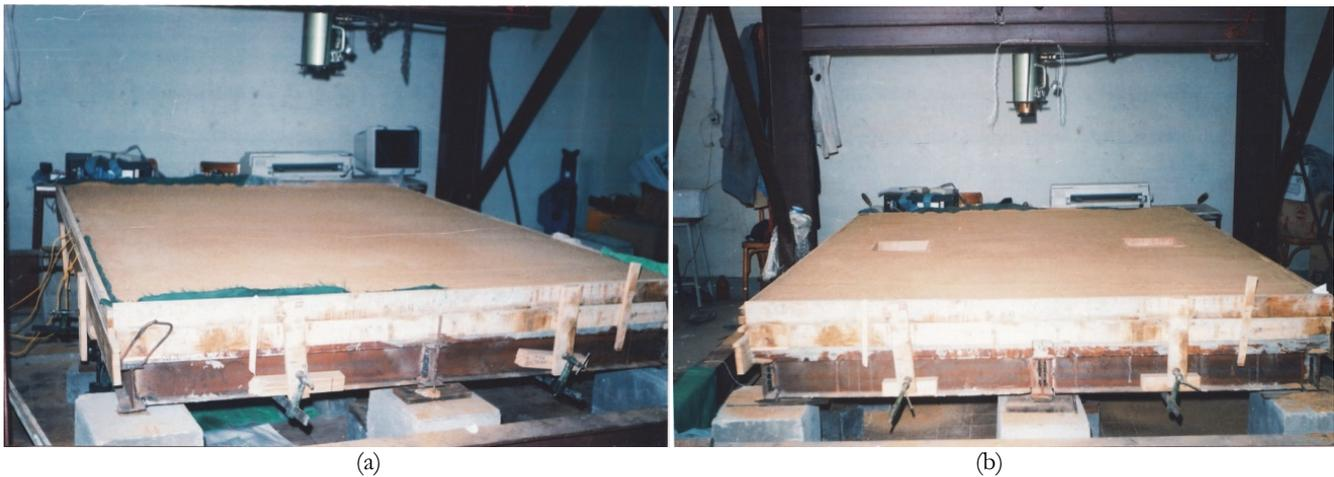
Figure 13: Final state of sand layers application (uniform distributed load). (a) Uniform load (M1); (b) Uniform load (M2).
