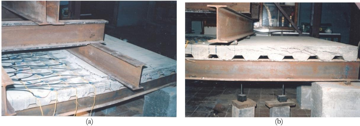
Figure 34: Failure mode and cracks pattern for reference model M1. (a) Perspective view; (b) Profile.
