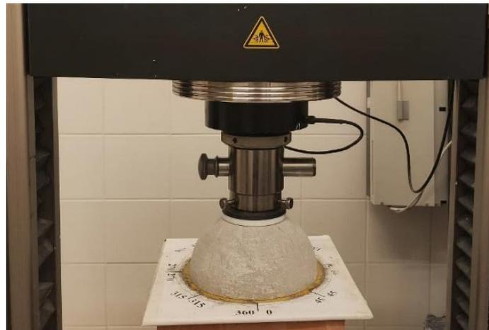
Figure 5: A specimen placed into the testing machine. Observe the plastic spacer between the specimen and the head of the testing machine.
