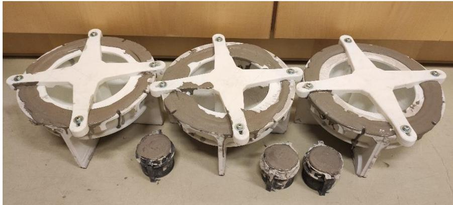
Figure 3: Preparation of the specimens. Dome molds and Brazilian Discs molds with the mixture inside, after vibration.
