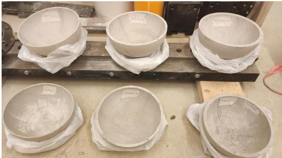
Figure 2: Some dome specimens after their removal from the mold.
