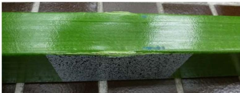
Figure 15: Failure mode of GFRP specimen.
