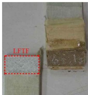
Figure 9: Failure modes of GFRP-GFRP single-lap joints: light-fiber-tear LFTF.
