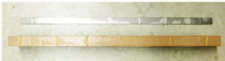
Figure 16: Failure mode of GFRP specimen reinforced with epoxy resin EPXRN and steel plate.
