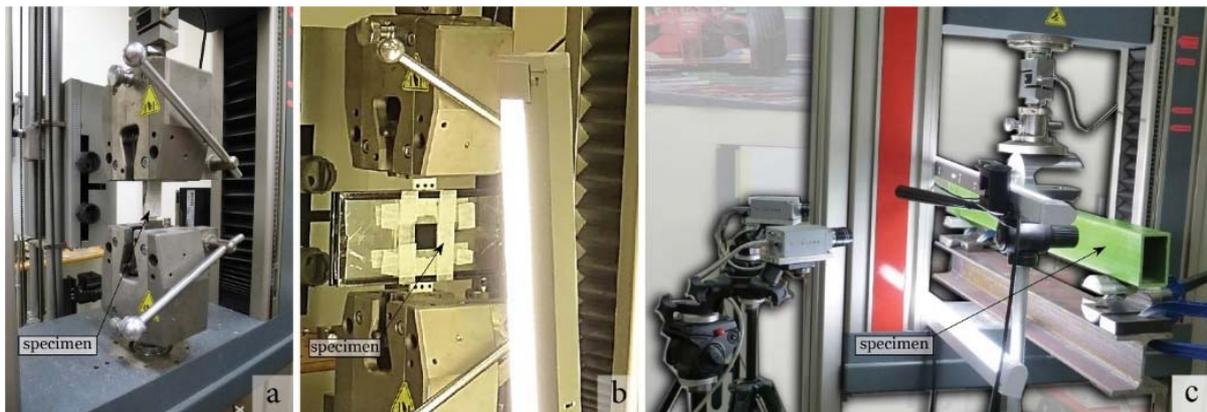
Figure 4: Experimental setup: shear test on GFRP-GFRP single-lap joints (a), shear test on GFRP-glass double-lap joints (b), bending test on GFRP steel squared tubular beams (c).
