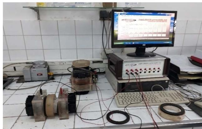
Figure 4: Device for Chloride diffusion test.
