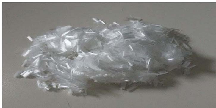
Figure 1: Polypropylene fiber (PP).
