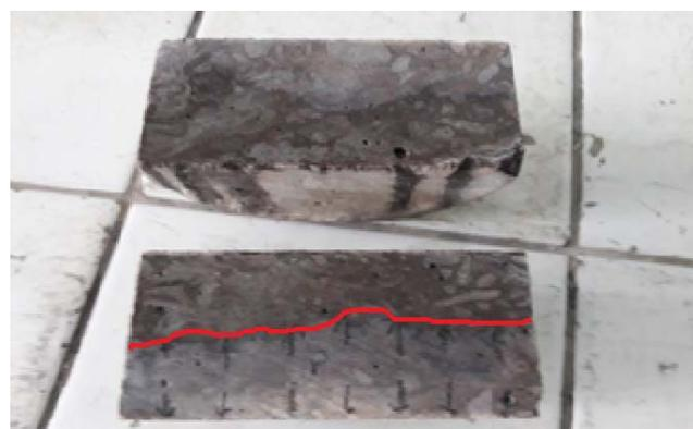
Figure 5: Depth of penetration of chloride ions in the sample.
