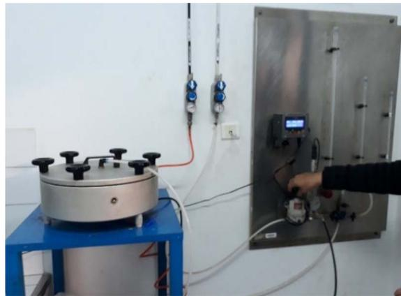
Figure 3: Inflation of the chamber to 8 bars and Measurement of oxygen permeability
