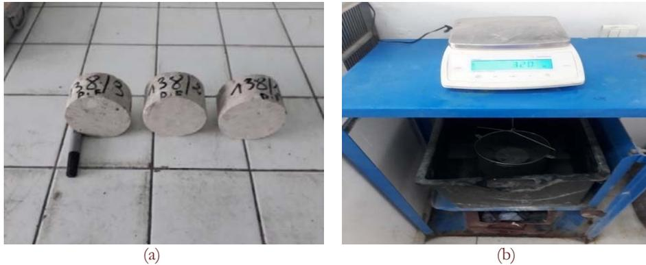
Figure 2: Porosity test (a) Three samples of the fiber-reinforced concrete (Ø100x 50 mm) prepared; (b) Weighing the sample
