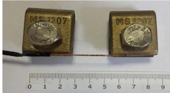
Figure 5: SC2 configuration, the grating is hanging between the two clamps.
