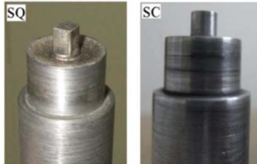
Figure 2: Friction stir welding tools with different pin profiles [13].
