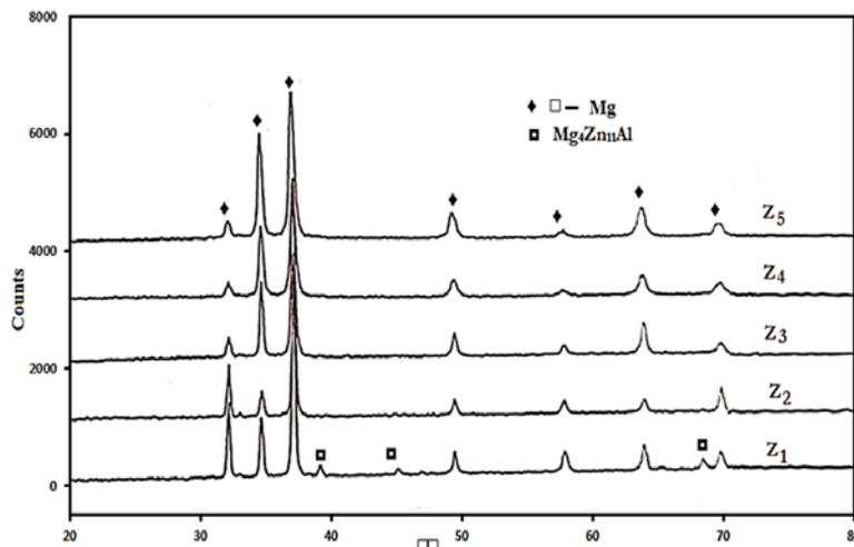
Figure 4: X-ray diffraction pattern of as cast and Solution treated samples
