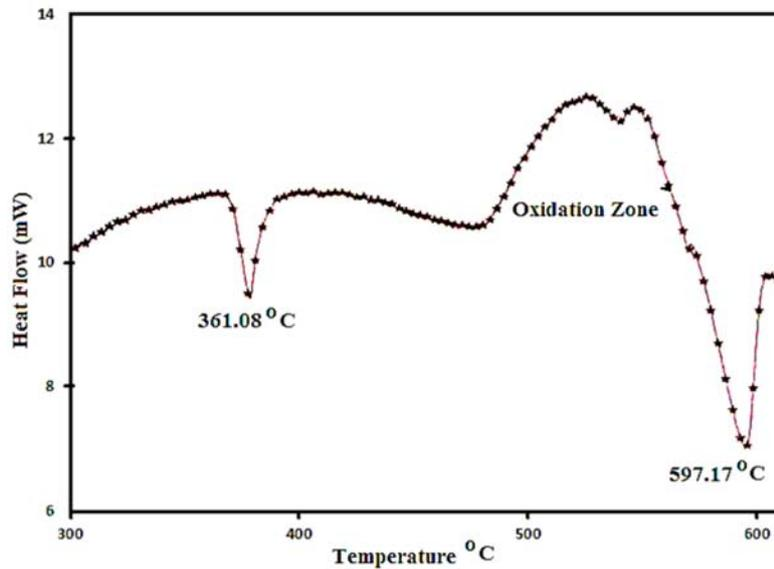
Figure 3: DTA thermograph (Heating rate of 10 °C min<sup>-1</sup>)
