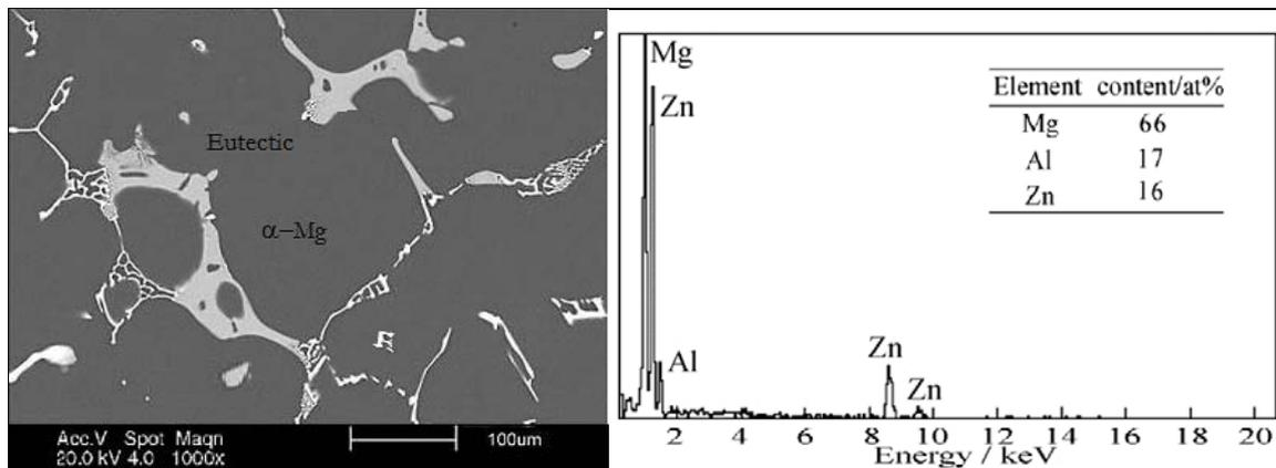
Figure 2: (a) SEM micrograph of as cast Mg-alloy (b) SEM-EDS of eutectic ternary phase
