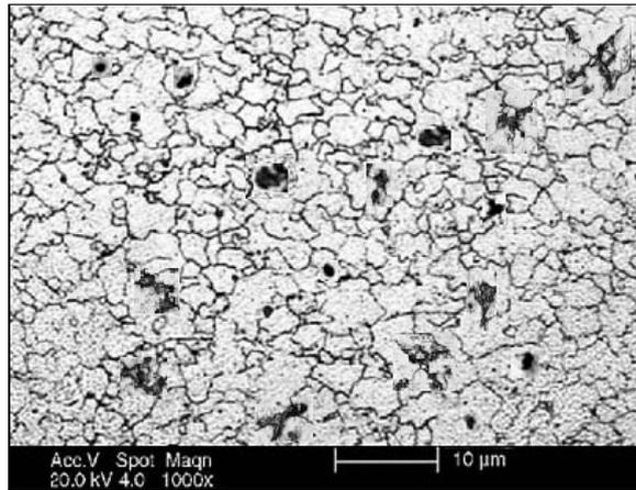
(c) Solution treated at 360 °C for 96 hours
