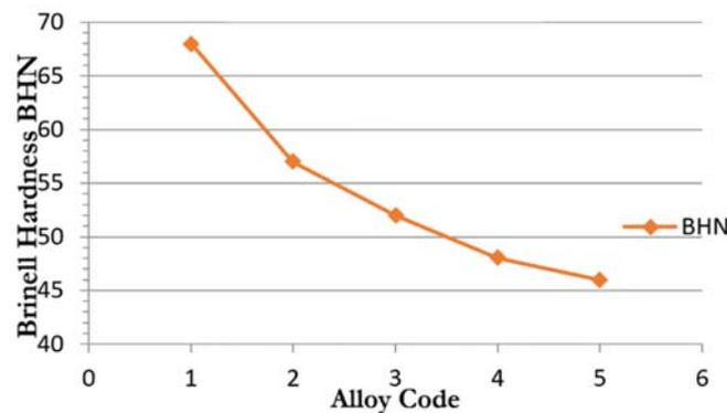
Figure 7: Brinell hardness for as Cast and ST samples
