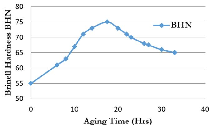
Figure 8: Hardness variation with different aging time
