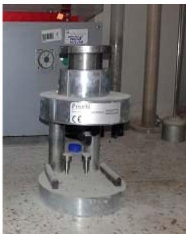
Figure 2: Tensile machine, three point bending test.
