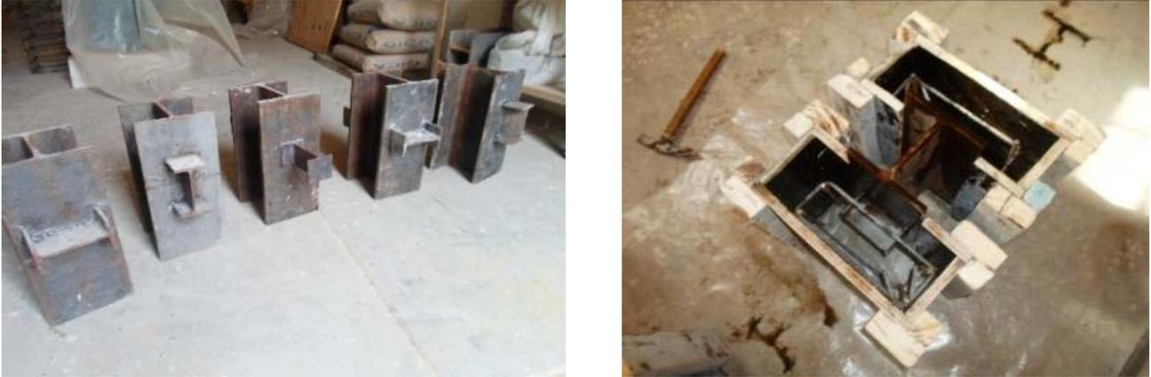
Figure 2: Push-out specimens' preparation.
