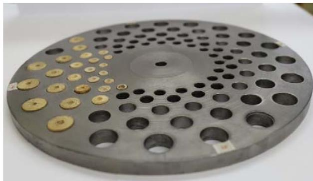
Figure 1: Model of bimetallic perforated plate.
