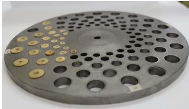
Figure 1: Model of bimetallic perforated plate.
