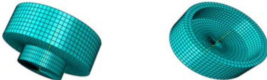
Figure 12: joint geometry and Mesh (contact zone)
