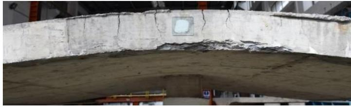
Figure 10: Crack distribution in the thickness direction on the long sides of the plate.
