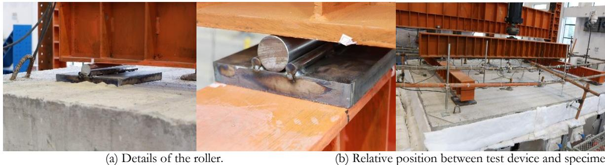
Figure 4: Details of the roller and relative position between test device and specimen.
