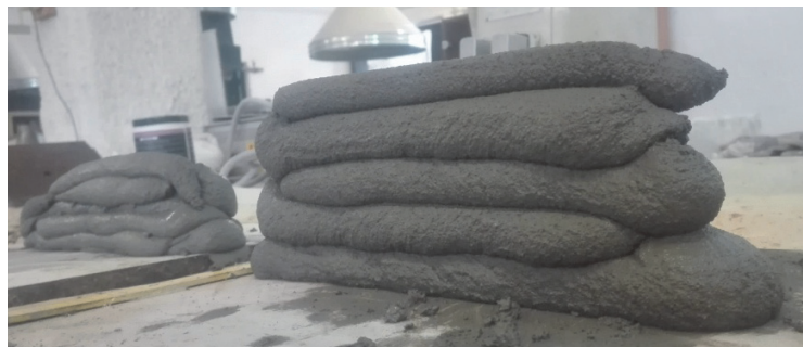
Figure 6: Difference on printing quality due to different workability of the same mixture 0 (left) and 15 minutes (right) after mixing.
