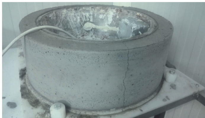
Figure 2: Formation of crack on concrete due to restrained shrinkage.
