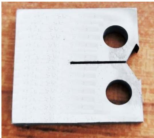
Figure 1 (a): CT Specimen with 780°C IQ temperature
