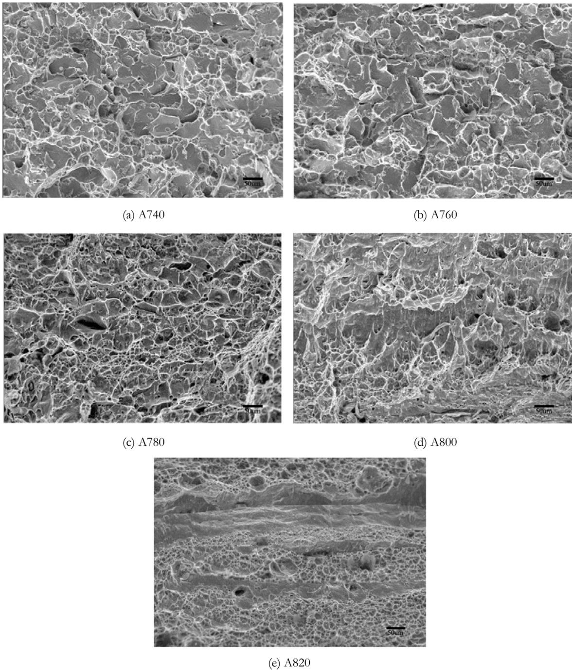
Figure 3: Microstructure of fractured surfaces for DP steels
