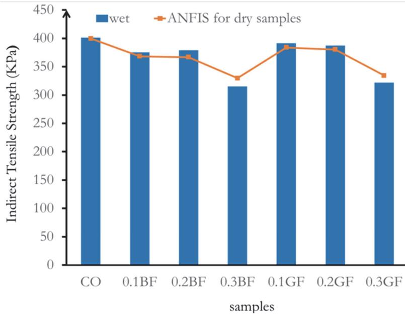
Figure 7: Indirect tensile strength results for wet condition.
