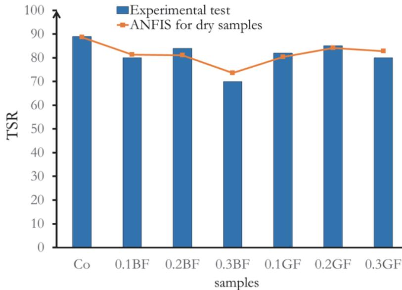
Figure 8: Tensile strength ratio (TSR) of control and fiber-reinforced samples.
