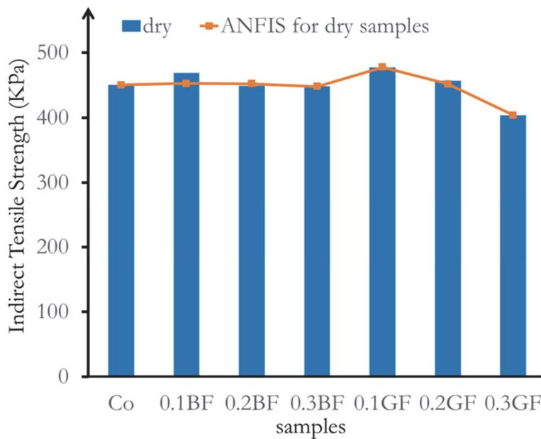
Figure 6: Indirect tensile strength results for dry condition.
