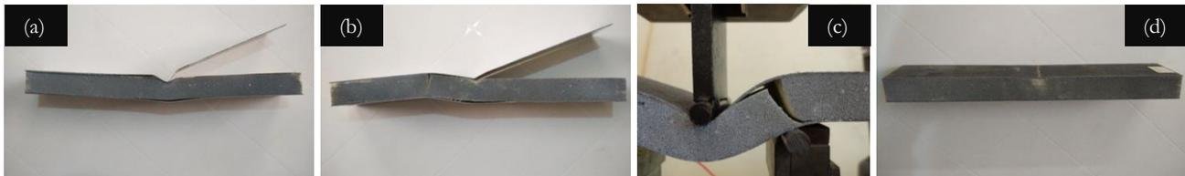
Figure 9: Failure behavior of sandwiches under 3PB tests: (a) *SA\_short\_3PB*; (b) *SA\_long\_3PB*; (c) *SB\_short\_3PB*; (d) *SB\_long\_3PB*.
