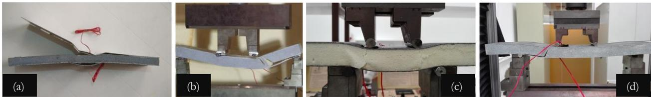
Figure 10: Failure behavior of sandwiches under 4PB tests: (a) *SA\_short\_4PB*; (b) *SA\_long\_4PB*; (c) *SB\_short\_4PB*; (d) *SB\_long\_4PB*.
