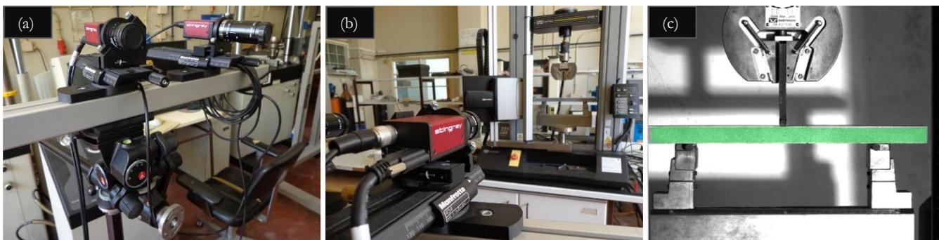
Figure 4: Digital Image Correlation with VIC2D system: (a) Cameras installation; (b) Image capturing (c) AOI.
