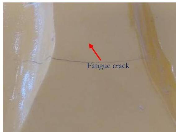
Figure 5: Fatigue failures on moving arm of No.2 excavator, which is the same as failure position of No.1 excavator
