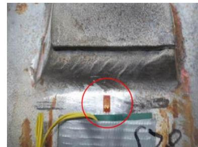
(a) Strain gauge measuring point
