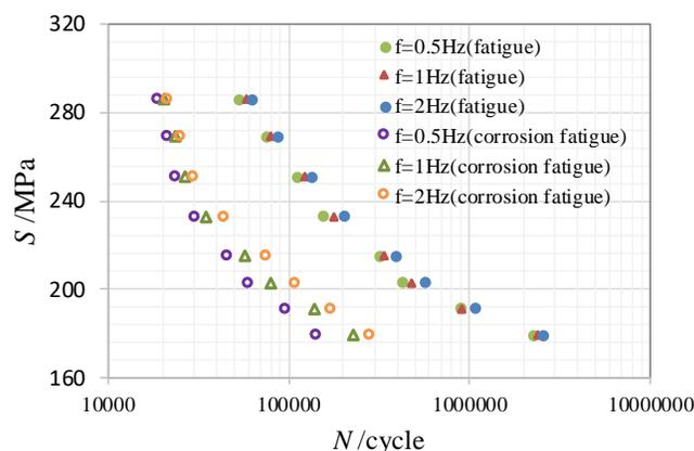
Figure 3: Results of fatigue and corrosion fatigue tests.
