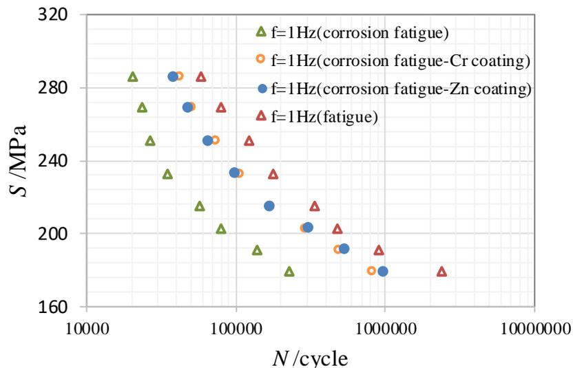
Figure 6: S-N curves of corrosion fatigue tests
