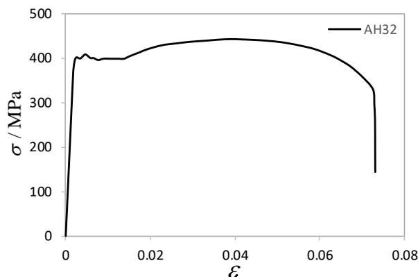
Figure 1: Stress-strain relation of AH 32 steel.
