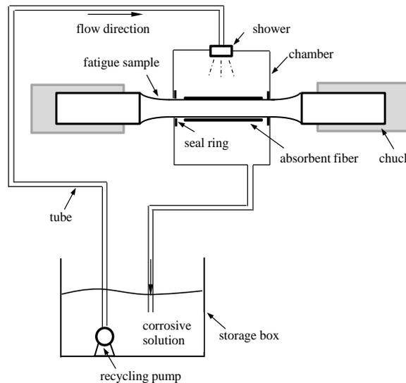
Figure 2: Setup of circulation device of corrosion solution.
