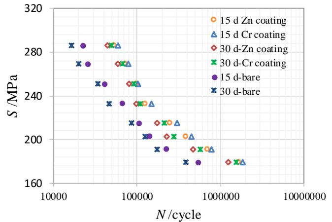
Figure 8: S-N curves of corrosion fatigue.
