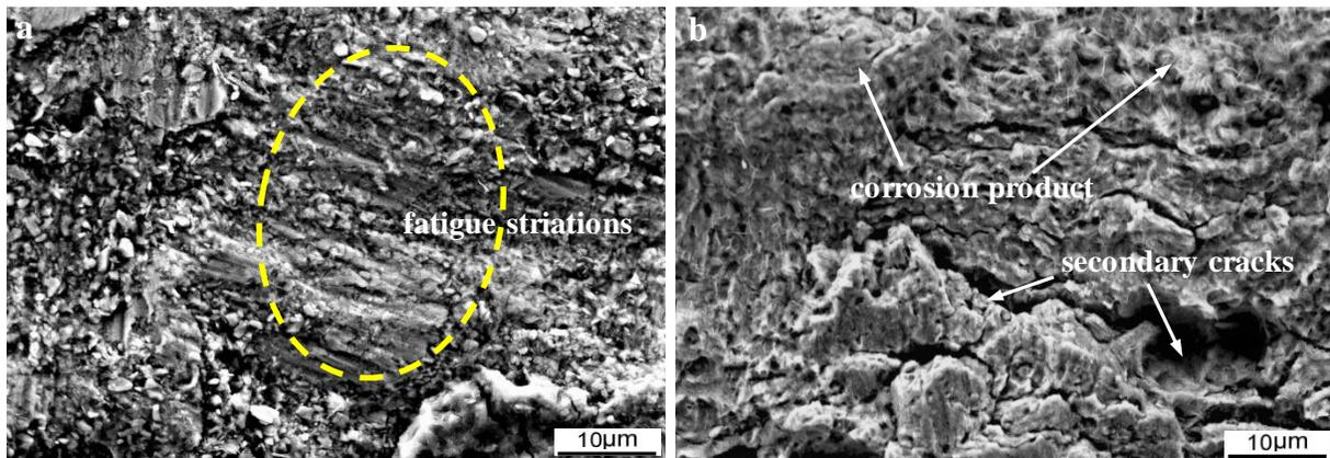
Figure 10: Morphology of crack propagation zone (a. Zn coating, b. Cr coating).
