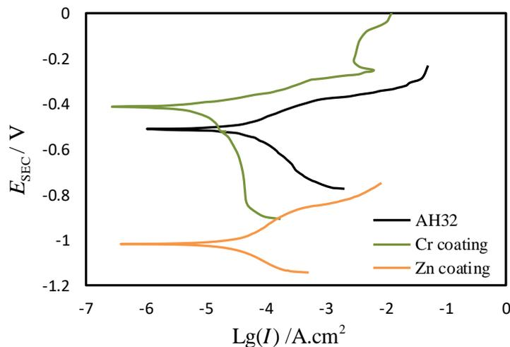
Figure 9: Tafel polarization curves of coatings and substrate
