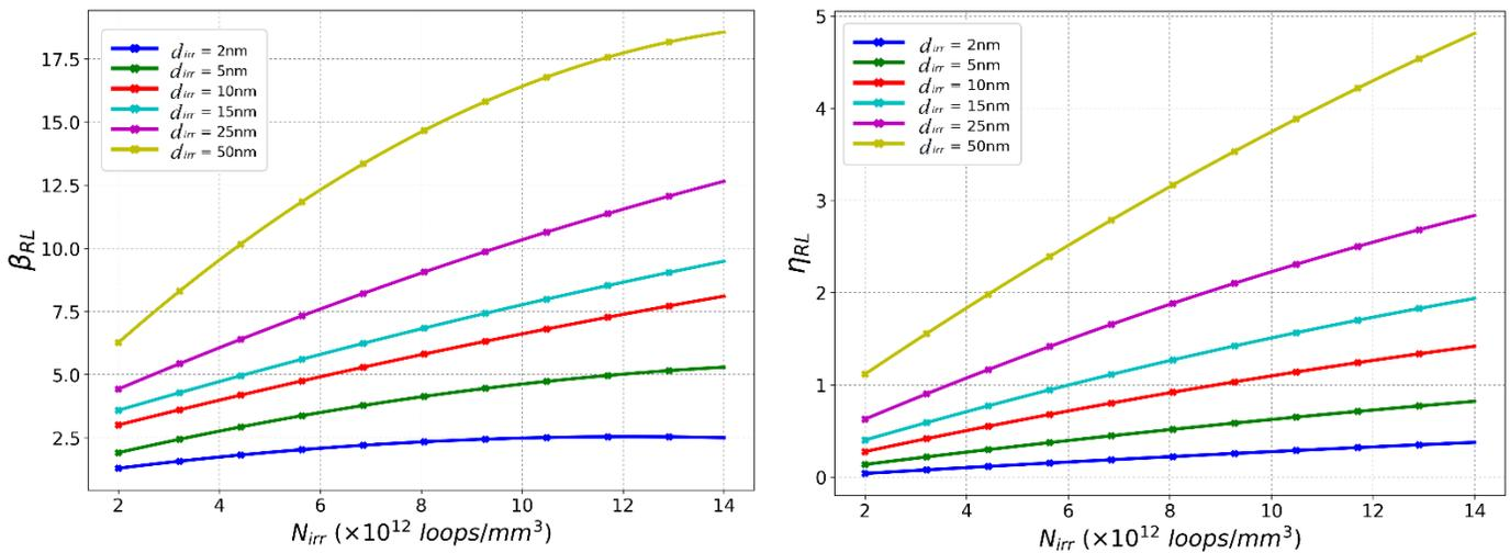
Figure 4: Relative change in Weibull distribution parameters for different irradiation defect size and number density. Subscript 'RL' represents the relative value of the corresponding parameter. For example, the relative change in the shape parameter is defined as  $(\beta_{irr} - \beta_{non-irr}) / \beta_{non-irr}$ .
