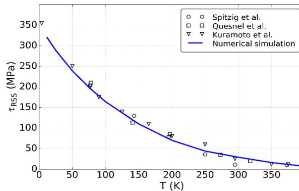
Figure 1: Validation of a material model with experimental results: resolved shear stress variation as a function of temperature.
