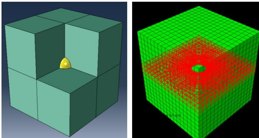
Figure 2: Unit cell model with inclusion, the meshed model with a highlighted area of consideration for Weibull distribution's parameter estimation
