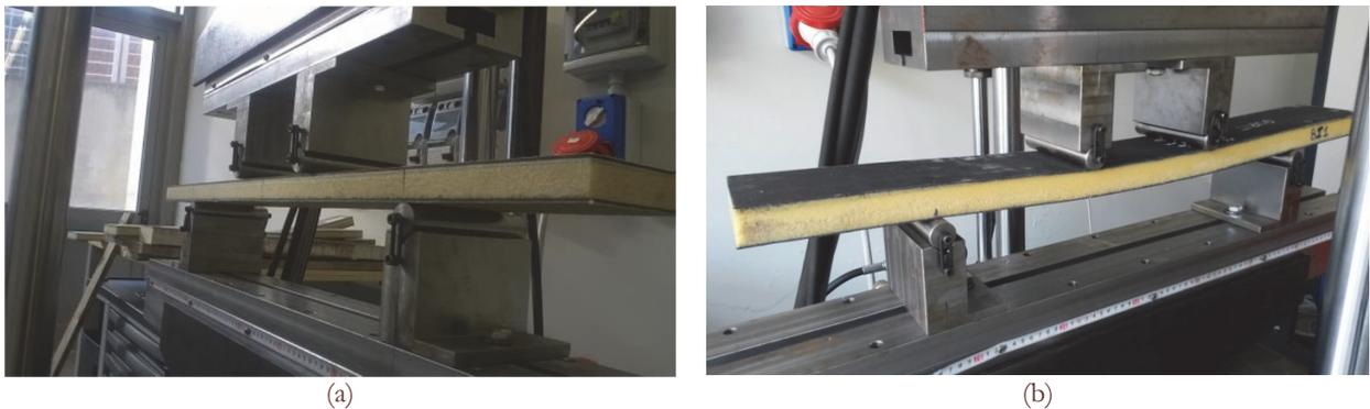
Figure 7: Initial set up for the A sandwich (a) and B sandwich (b).
