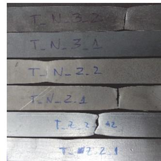
Figure 5: Conventional stress-strain curves of two steel grades under investigation (S355MC and S350GD). Detail shows the yield zone of the steel grades (left). Aspect of the specimens tested (first four (symbol N) are S355MC and last two (symbol Z) are S350GD).
