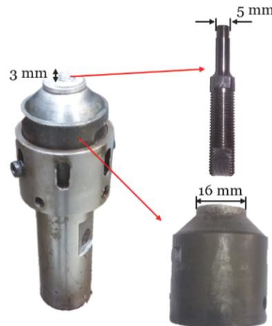
Figure 10: FSW tool used
