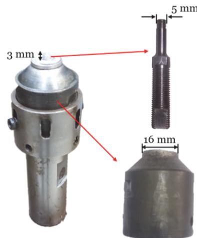
Figure 10: FSW tool used
