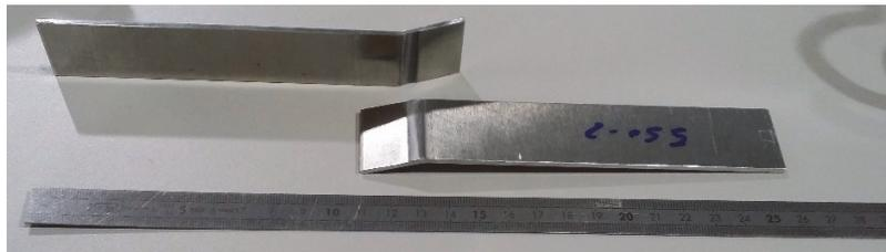
Figure 24: Fracture mode I in SLJ joints FSW\_550-1 of with 550 kgf downward force
