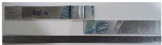
Figure 22: Different views of mode II failure in a joint
