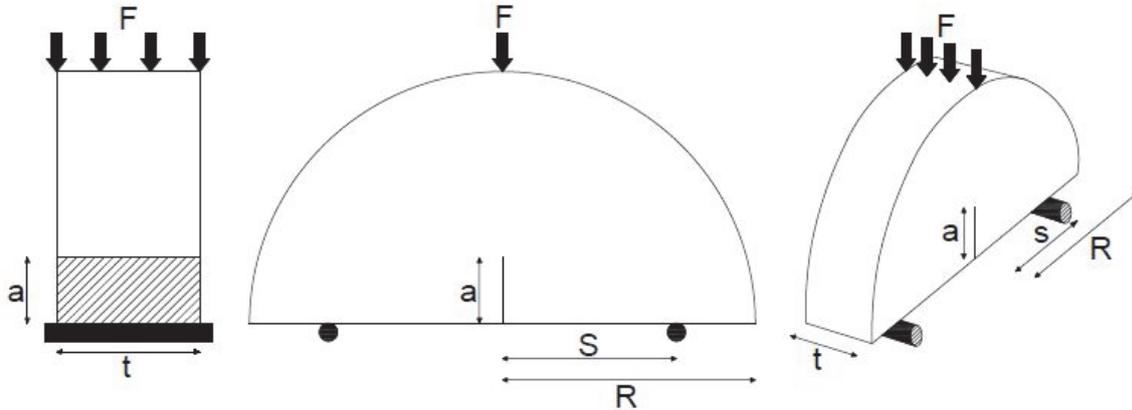
Figure 2: Schematic view of edge cracked SCB specimen under mode I loading.
