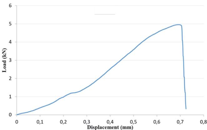
Figure 8: A load-displacement curve obtained for the SCB test sample modified with EPS 15.
