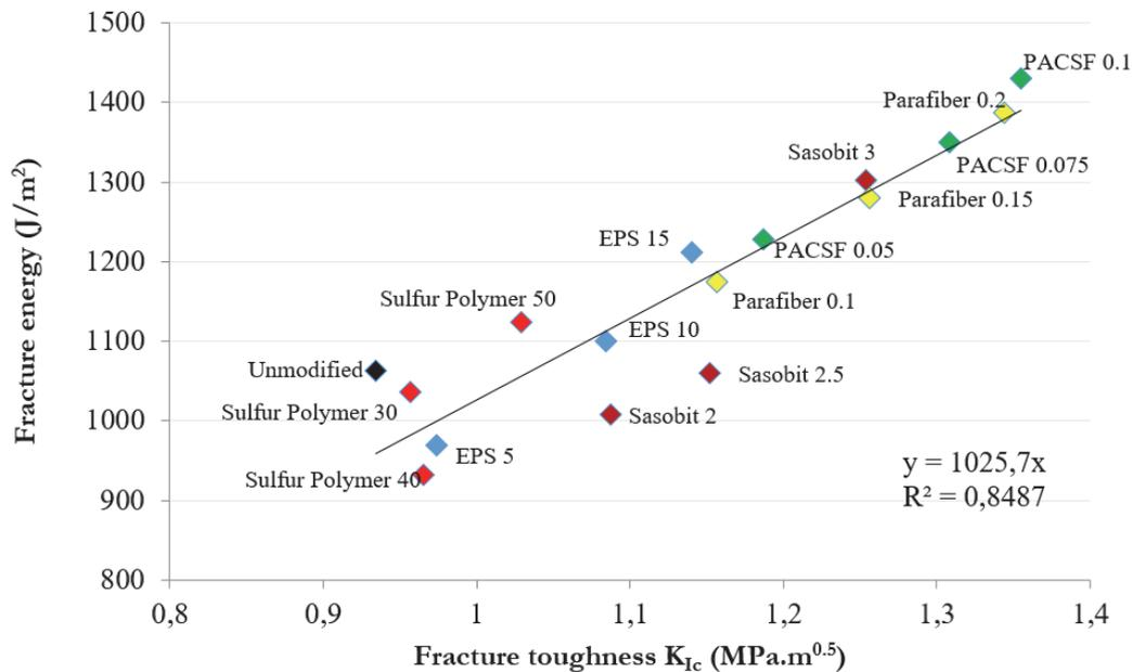
Figure 12: The relationship between the observed average fracture energy and fracture toughness of modified and unmodified asphalt mixtures.
