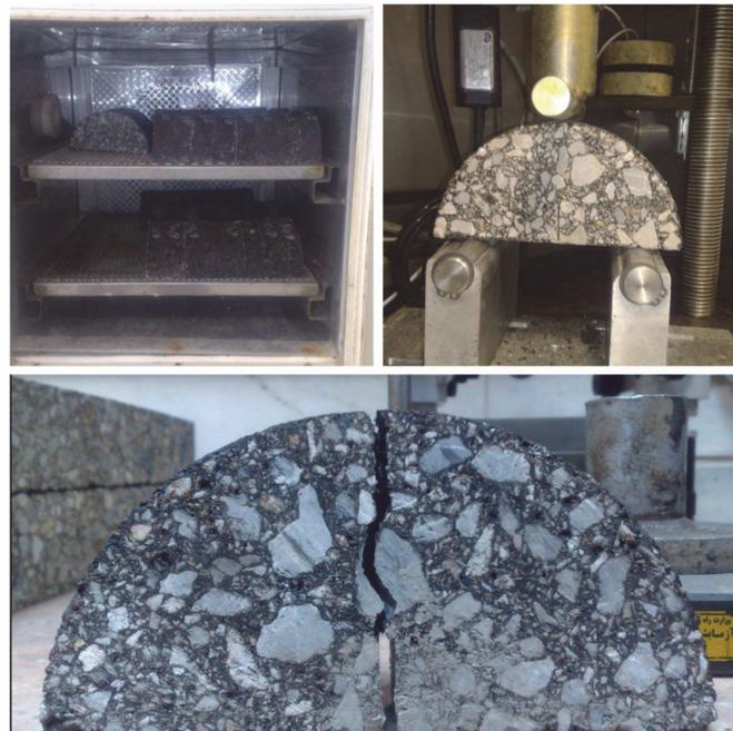
Figure 3: Crack propagation testing process.
