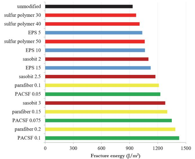
Figure 10: Bar chart of average fracture toughness of specimens.
