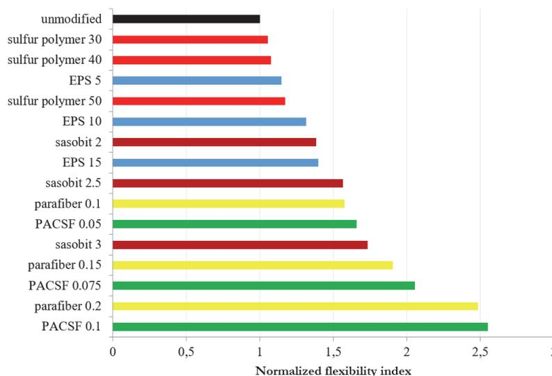
Figure 13: Flexibility Index of modified asphalt mixtures, normalized in relation to the unmodified mixture
