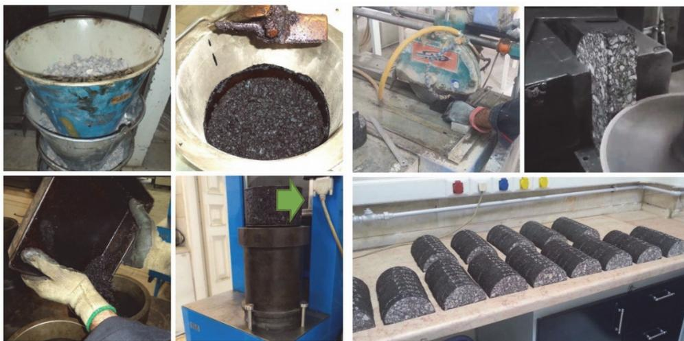
Figure 1: Steps involved to produce edge cracked SCB specimens.
