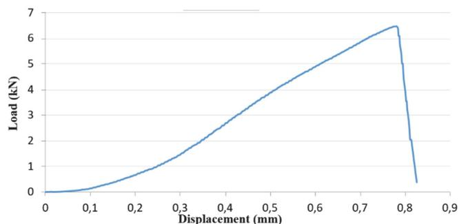
Figure 9: A load-displacement curve obtained for the SCB test sample modified with Parafiber 0.2.
