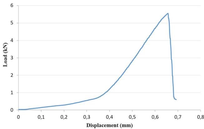
Figure 6: A load-displacement curve obtained for the SCB test sample modified with Sulfur 50.
