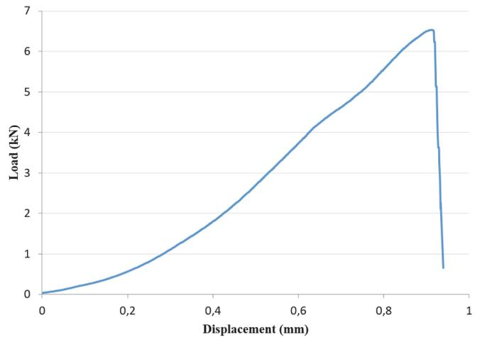
Figure 7: A load-displacement curve obtained for the SCB test sample modified with PACSF 0.1.
