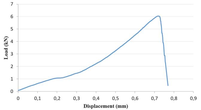
Figure 5: A load-displacement curve obtained for the SCB test sample modified with Sasobit 3.
