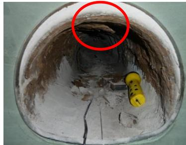
Figure 21: Failure in the model overload test.
