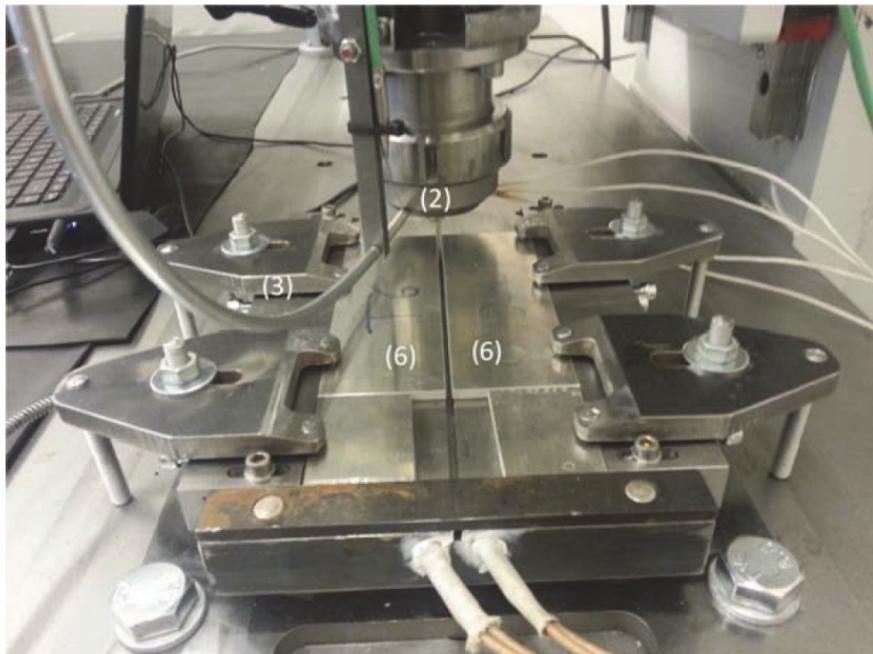
Figure 29: Experimental setup of Al-Al HYB configuration: HYB spindle extruder (2), steel fixture (3), and aluminum plates to be welded (6).
