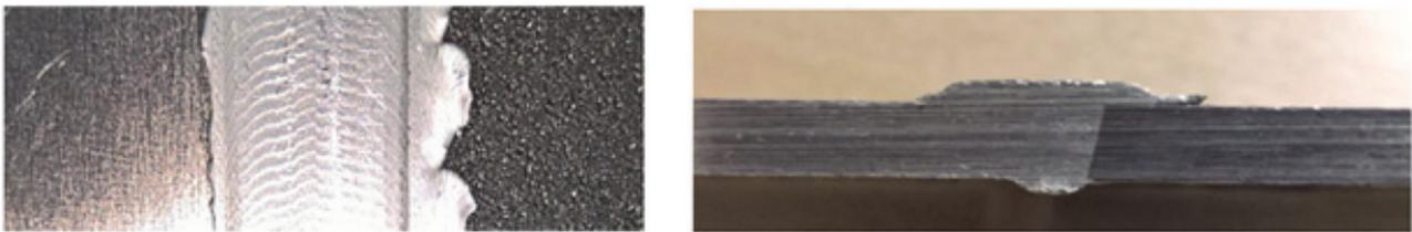
Figure 32: Upper and transversal appearance of HYB dissimilar welded plates. Aluminum on left side, steel on the right side.
