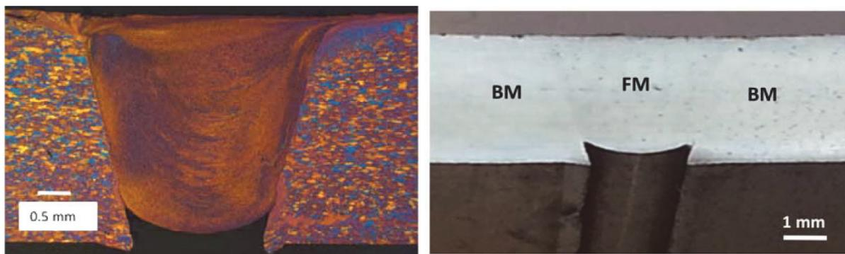
Figure 30: Optical macrograph of the joint cross section.
