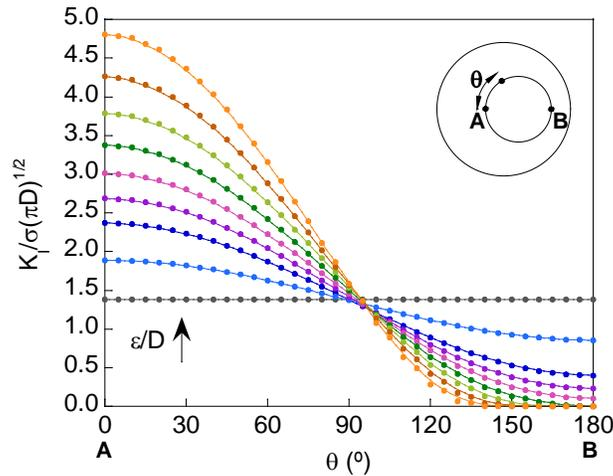
Figure 4: Dimensionless SIF along the crack front for  $d/D=0.4$  and  $\varepsilon/D$  from 0 to 0.200 with increments of 0.025.
