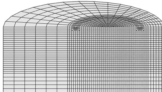
Figure 1: 3D mesh of the bar with a non-symmetric annular crack.
