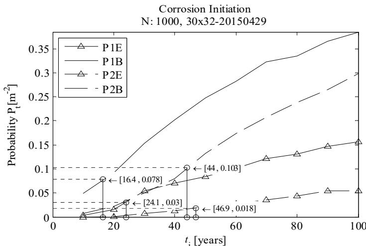
Figure 4: Probability of corrosion initiation  $t_i$  for the variants considered by type of reinforcement protection. B - unprotected reinforcement, E - epoxy-coated steel reinforcement; and the bridge deck type. 1 - directly exposed bridge deck with a crack, 2 - ordinary concrete and a bridge deck with a crack protected by waterproof insulation under an penetrable asphalt overlay.
