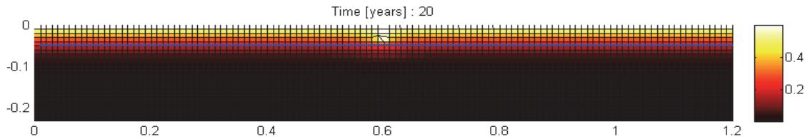
Figure 2: The sample contour plot of concentration of chloride ions in a concrete bridge deck with a crack. Deterministic solution for an exposure period  $t = 20$  years shows the FEA meshed elements and concentration in the form of contours.
